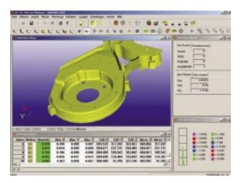
"3D-Tol" is the ideal program for comparing the measurement data from three dimensional surfaces, to the nominal data supplied in the form of a CAD model. Typically it is used for automotive body parts, but increases in 3D machining capabilities make it applicable to many applications in aerospace, marine and consumables engineering.
